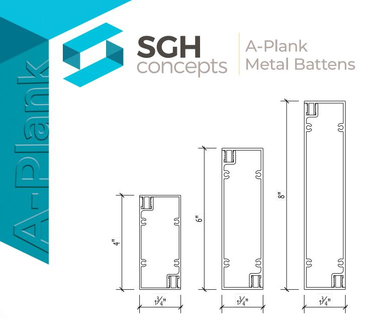
Constructed with minimum .080" aluminum, A-Plank Battens can be installed vertically or horizontally and are a complement to the building. A-Plank Batten's simple design allows for ease of detailing and installation to get it on the building quick and easy.
